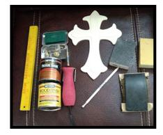
Step 1: Prepare wood product by sanding the finish off with both a coarse and fine sand paper.
